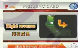
The left DC motor moves backward and right DC motor stop.
