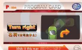
The left DC motor moves forward and right DC motor stop to make the model turn right.
