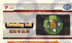
The left DC motor moves backward and right DC motor moves forward to make the model turn as anticlockwise.
