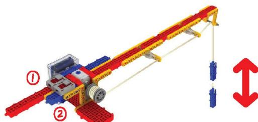
Press touch sensor 1, 2, the fishing-rod will move up and down.
